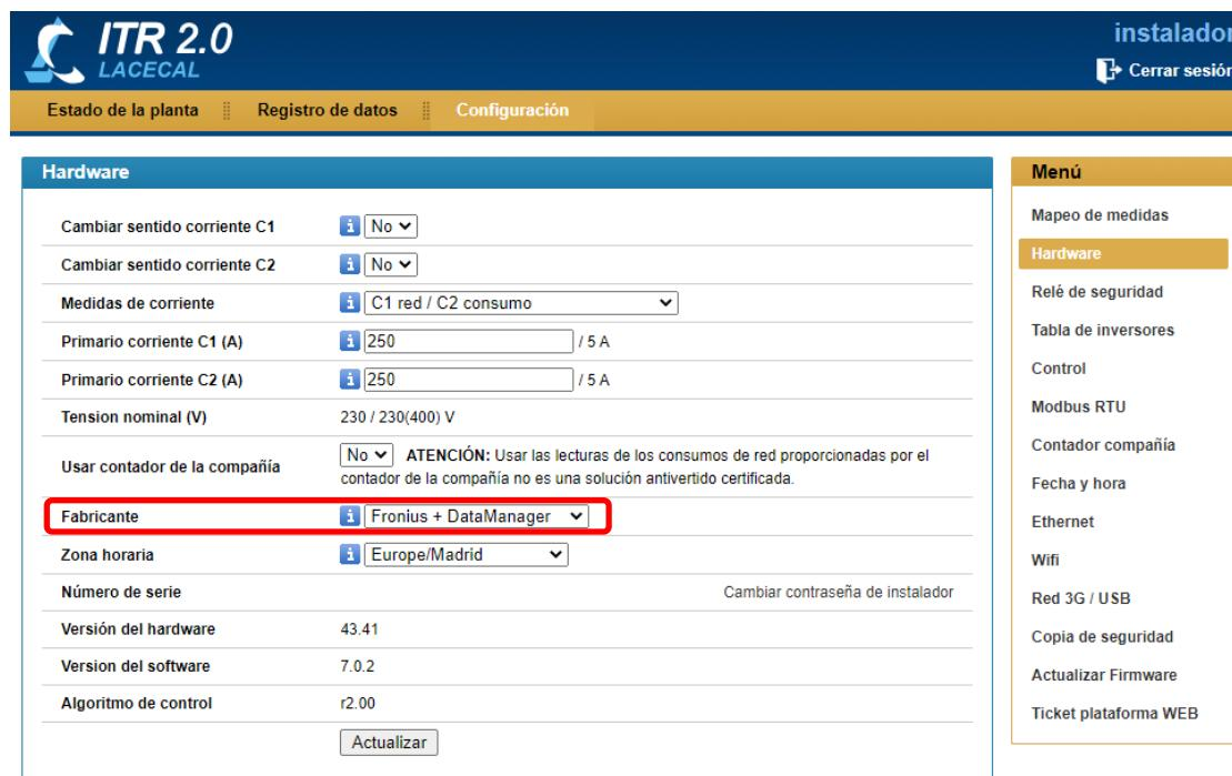
The screenshot shows the 'Hardware' configuration page. The 'Fabricante' dropdown is set to 'Fronius + DataManager'. A note below it states: 'ATENCIÓN: Usar las lecturas de los consumos de red proporcionadas por el contador de la compañía no es una solución antivuelto certificada.' (Attention: Using the readings of the grid consumption provided by the company meter is not a certified anti-tampering solution.)
