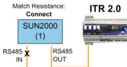
If there are several inverters, they will be connected in cascade as shown in the following figure. In the inverter located at the opposite end to the ITR the 'Match Resistance' option will be set to 'Connect', and in the rest of the inverters to 'Disconnect' (If this option is available).
