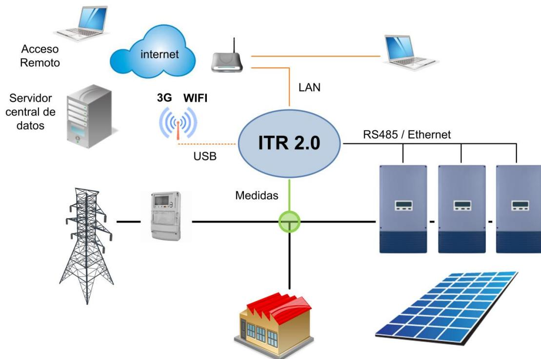
The mains voltages are connected directly, while external current transformers with 5 A or 250 mA secondary are used for current measurement. The power measurement accuracy of the ITR is 1%.
